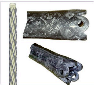
Fig.5: Winding the tube together with the interface shapes
