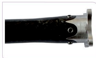
Fig. 6: Torque shaft assembled without adhesive
